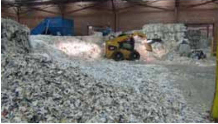
Sustainable communities recognize environmental and economic benefits of a zero waste society. Communities that embrace recycling often are home to Material Recovery Facilities (MRF). In this photo from an Asheville, NC “clean MRF” operated by American Recycling, a skid-steer readies recycled paper for baling before transport to a nearby paper mill.
